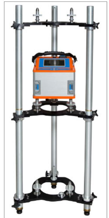
**The CG-6 Autograv™ is the next generation land gravity meter combining a modern, intuitive user interface with our renowned quartz sensor technology housed in a rugged yet lightweight enclosure.**
