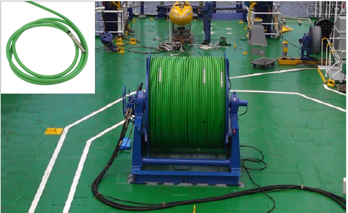
**The GeoEel Solid digital hydrophone streamer is the smallest diameter solid design available.**
