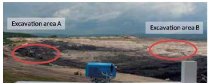
The maximum distance was set to 1500 m, with a range resolution of 0.5 m and azimuth resolution of 5.4 mrad. The displacement is close to zero in almost all the area except in one part where a deformation of about 100 mm appears, this is due to the excavation works.
